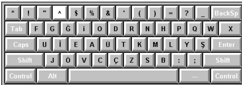
Turkish-F Type (AltGr State) - Also Shift + AltGr State to get CAP AE ligature
